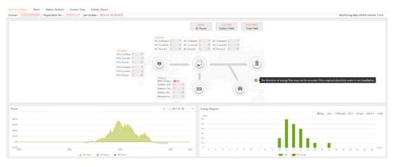
b. Battery Analysis. It contains the data curve and battery status. Please note that [Battery Information] shows the total data of all batteries used in an inverter.
